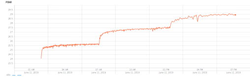
Figure 2: PSNR calculated on validation dataset during training. The steep jumps in the curve correspond to addition of the higher resolution module to the network.
